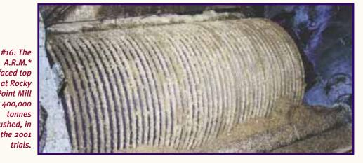
A.R.M.\* Hardfaced top roll at Rocky **Point Mill** after 400,000 tonnes crushed, in the 2001
